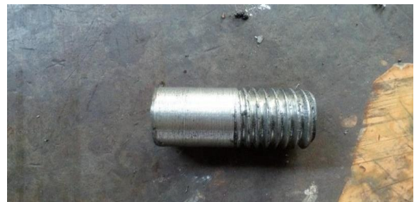
Fig-7: Drive shaft coupling finger (as a work piece)
